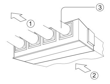
\* Air outlet \* Air inlet \* Ventilation hole
